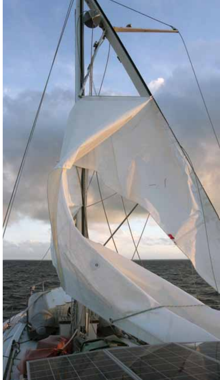
The crew of Brick House waited until morning to begin the tricky process of removing the mainsail after a stainless-steel chainplate failed, causing the mast to snap.
