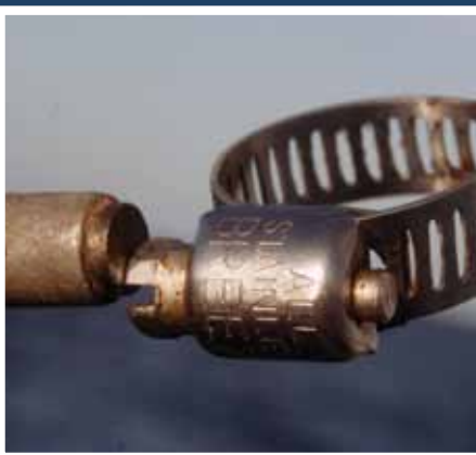
Some poor sailors still fall victim to the common “stainless-steel” hose clamp with a mild steel screw.
