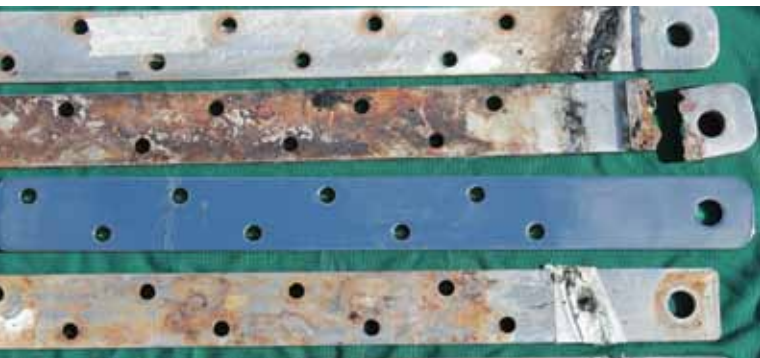
The new titanium chainplate shines brilliantly among the stainless steel ones it replaced, including the one that broke.
